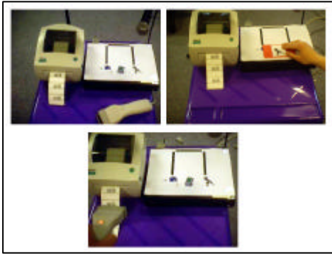
Figure 4. Using RFID tags to record sound and associate them with barcodes which can be placed on top of pictures. The scanned pictures can then be used to retell a story (with sounds) via barcode readers.
