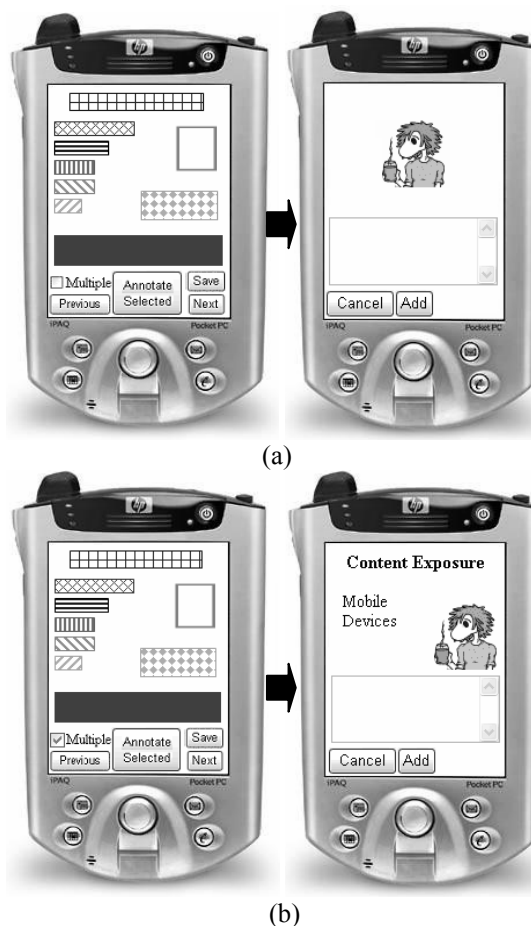
Figure 6. Using the image map to display selected content. The representation corresponds to the slide shown in Figure 3a. (a) The results of selecting a single content block. (b) The results of using multiple select to select numerous content blocks.
