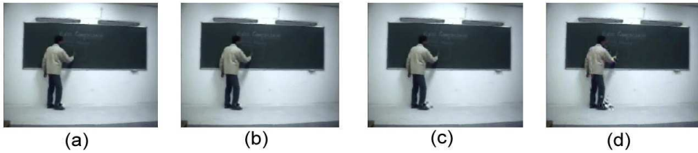
Figure 6. Reconstructed frames for a GOP (a) frame 21 (I frame), (b) frame 22, (c) frame 24, (d) frame 28 at 0.6 bpp without segmentation and bandwidth allocator.
