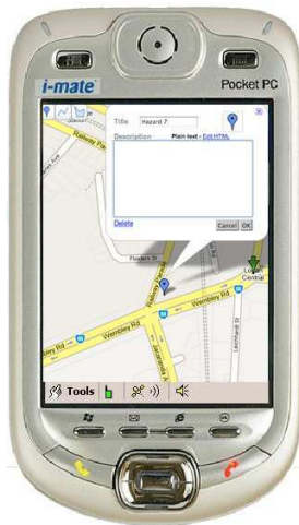
Figure 2. Digital field journal: interactive road map with participant-inserted road hazard identifier, tagged with risk assessment entry.
