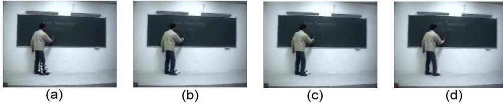
Figure 13. Reconstruction of frame 24 at (a) 0.1 bps (b) 0.2 bps (c) 0.3 bps (d) 0.5 bps with bandwidth allocator and segmentation
