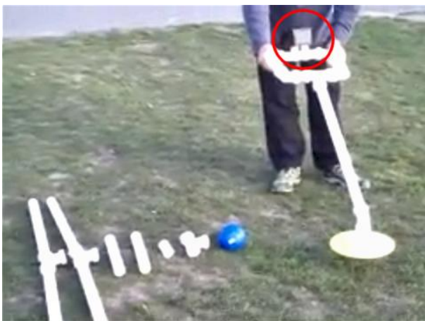
Figure 4: Mock-up metal detector composed of lightweight waste pipes. The smartphone is embedded into an open box attached to the tool handle (circled)
