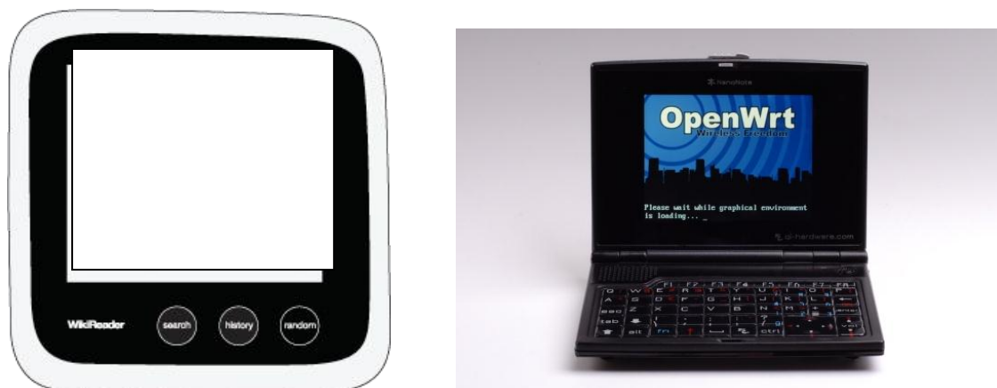
Figure 1a. Wikireader – offline handheld reading device. Figure 1b. Ben Nanonote - an ultra small form factor copyleft computing device which has 336 MHz XBurst CPU, 3.0” display and 2GB NAND flash memory.
